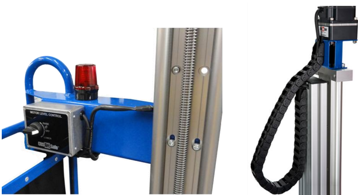
Figure C-1: Power slide components including the power slide control box and motor
