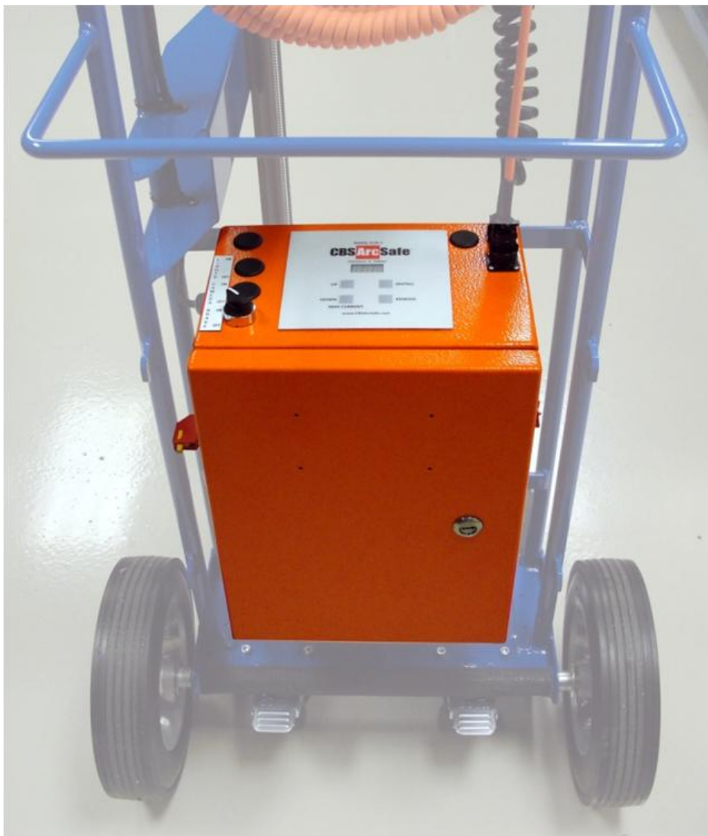
Figure 3-11: RRS-1 Control cabinet
