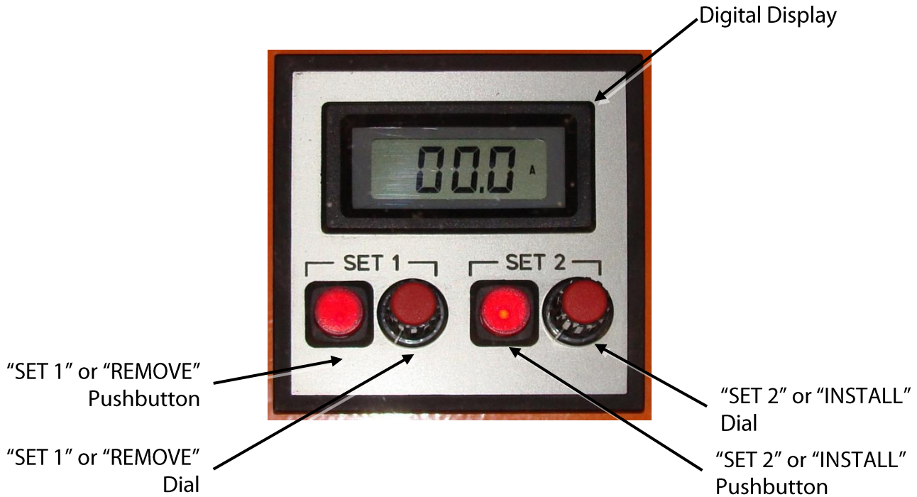
Figure 3-4: CBS ArcSafe® Legacy CCM configuration
