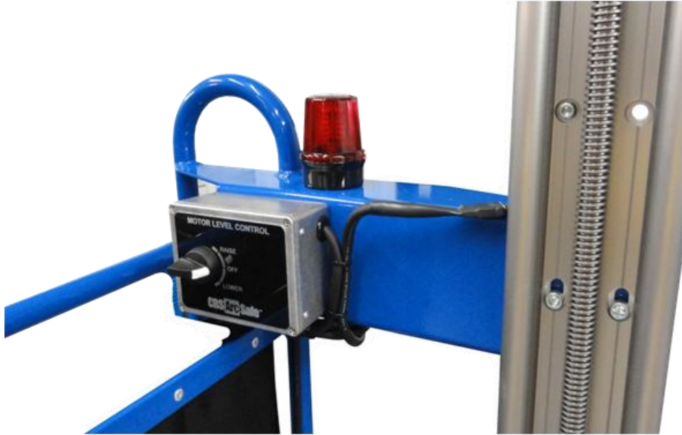
Figure 1-20: CCM Status Indicator Light
