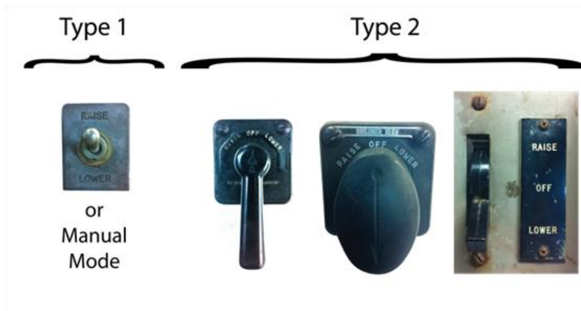
Figure I-4: Factory elevating motor switches
