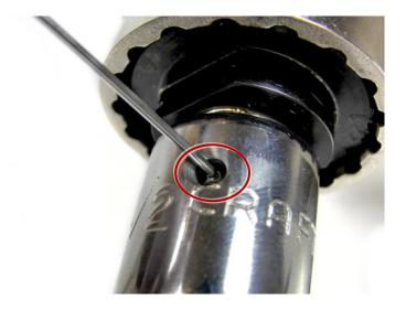
2. On the de-energized and OPEN test breaker, extract the breaker's racking handle, and fit the racking adapter to the handle as shown in the Installation section of this manual.
