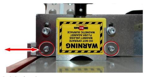
3. Re-tighten the bolts after adjustment.
