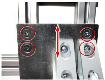
2. Slide the motor up or down to achieve proper alignment with theracking mechanism of the breaker. Ensure that the drive motor and tool on the RRS-3 mates properly with the racking mechanism on the breaker.
