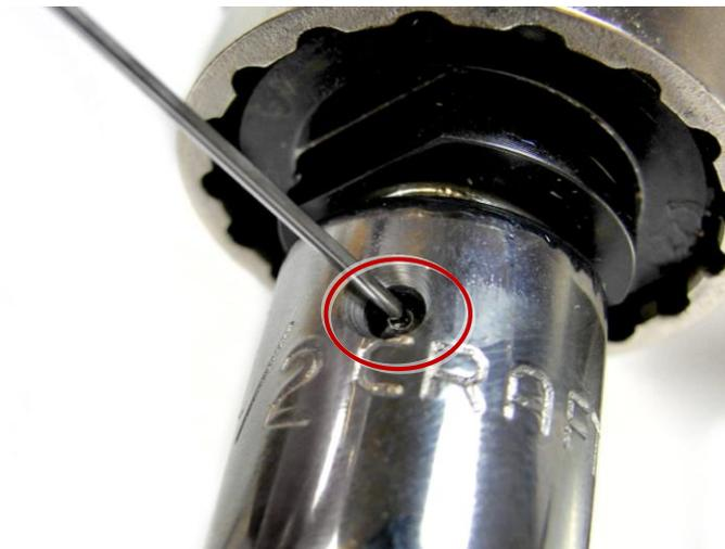
2. On the de-energized and OPEN test breaker, extract the breaker's racking handle, and fit the racking adapter to the handle as shown in the Installation section of this manual.
