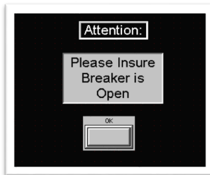
Figure 5: Breaker status safety prompt
