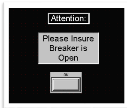
Figure 10: Breaker status safety prompt
