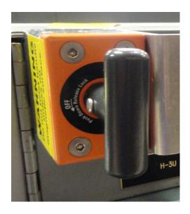
**Step 3**: Engage the magnet by turning the handle to the ON position.
