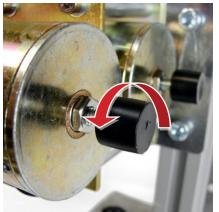
2. To decrease the solenoid plunger depth, loosen the nut on the solenoid plunger, and turn the black end clockwise. Test the depth by operating the appropriate plunger with the RSO, and re-tighten the nut.
