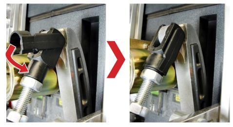
8. Manually push the charging arm back to its resting position before beginning operation. The RSA is ready for remote operations.
