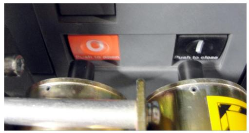
6. Place the charging arm adapter, removed in step 2, over the charging arm of the breaker. To do this pull out the charging arm slightly and slide the adapter over the arm.
