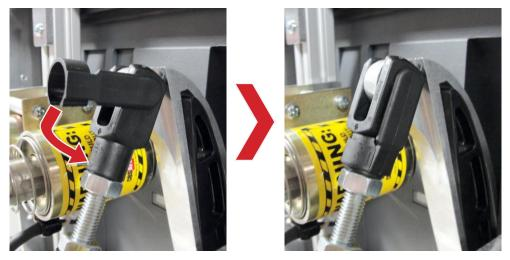
8. Manually push the charging arm back to its resting position before beginning operation. The RSA is ready for remote operations.
