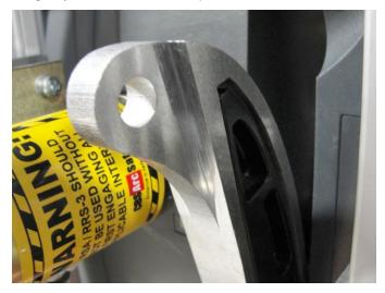
7. Reconnect the charging arm adapter to the RSA-120 using the clevis pin from step 2.
