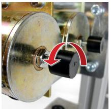
2. To decrease the solenoid plunger depth, loosen the nut on the solenoid plunger, and turn the black end clockwise. Test the depth by operating the appropriate plunger with the RSO, and re-tighten the nut.
