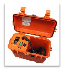
Step 3: Remove the cable from the cord storage area inside the RSO and connect the cable to the corresponding receptacle on the RSA-161A motor control box. Once the RSO-I AR has been connected, exit the arc flash boundary
