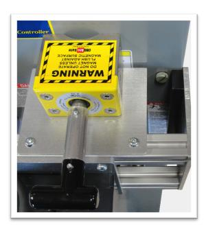
Step 4: Now, secure the RSA-161A into place using the twist lock magnet. Rotate the handle of the magnet 180° clockwise to engage the magnet and secure the RSA-161A to the equipment.
