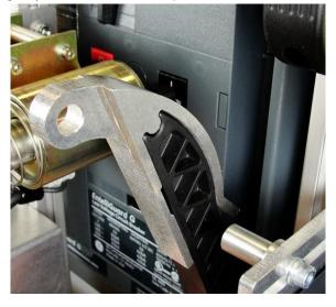
7. Reconnect the charging arm adapter to the RSA-120 using the clevis pin from step 2.
