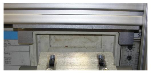
3. Turn the handles of the twst-lock magnets 180° clockwise to lock the RSA in place.
