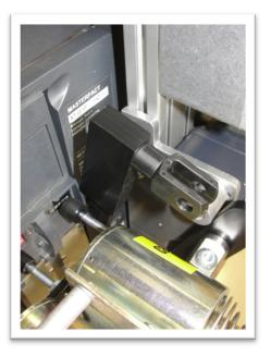
**Step 5**: Connect the charging linkage to the handle adapter by inserting the rod-end into the clevis and aligning the hole (Manual rotation of the motor arm may be necessary). Next, insert the clip through the rod-end and clevis and press the fitted end of the clip over the clevis to secure the linkage in place.
