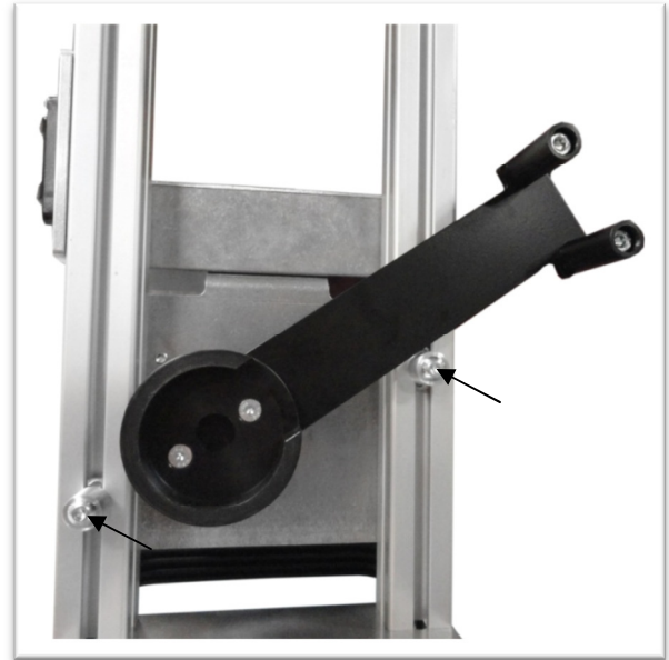
Figure 5: Loosen the bolt(s) indicated inside the stop(s) above to slide the stop(s) to the required location; after moving the stop(s) to the location needed, tighten the bolts back down to secure the stop(s) to the RSA-181
