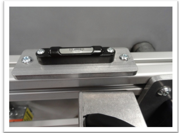
Figure 3: Use the built on leveler to ensure the RSA-181 is level with the breaker
