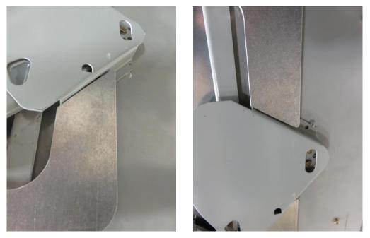
4. Turn the handles of the twist-lock magnets 180° clockwise to lock the RSA in place. Place the motor control box on the breaker so that the cord is free from moving parts.
