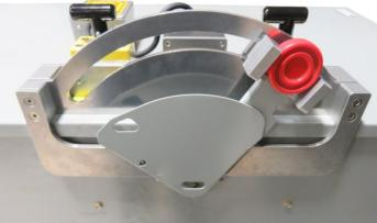
4. With the breaker in the OFF position, slide the OFF travel stop so it contacts the actuator arm, and tighten the bolt.
