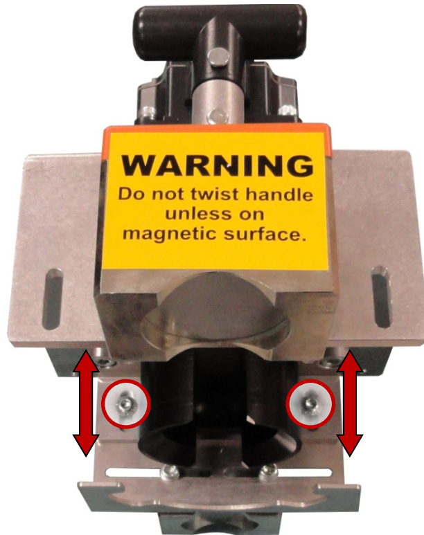
Figure 5 - Height adjustment on the top side of the RSA-34
