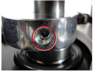
3. With the RSA operator arm in the OPEN position, rotate the outer limit switch cam until the limit switch is undepressed and clicks slightly, then rotate the cam back onto the switch until another slight click is heard, and the switch is depressed. Re-tighten the lock-screw on the cam.
