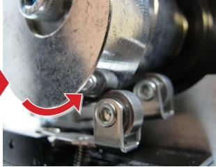
4. With the RSA operator arm in the CLOSED position, rotate the inner limit switch cam until the limit switch is undepressed and clicks slightly, then rotate the cam back onto the switch until another slight click is heard, and the switch is depressed. Re-tighten the lock-screw on the cam.
