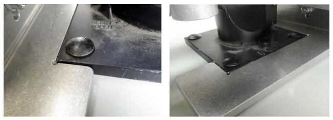
5. To attach the RSA to the breaker turn the handles of the twist-lock magnets 180° clockwise. The RSA is now ready for remote operation
