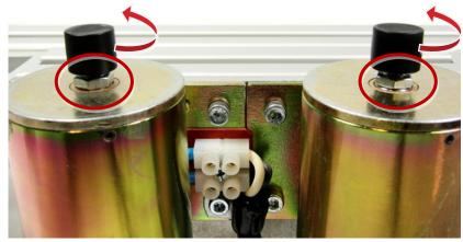
2. To decrease the solenoid plunger depth, loosen the nut on the solenoid plunger, and turn the black end clockwise. Test the depth by operating the appropriate plunger with the RSO, and re-tighten the nut.
