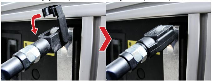
8. Manually push the charging arm back to its resting position before beginning operation. The RSA is ready for remote operations.
