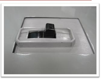
**Step 2:** Place the RSA-66A over the switch and secure the RSA into place by rotating the handle of the twist-lock magnet 180° clockwise. This will engage the magnet and fix the RSA to the panel as shown in the figure to the right.
