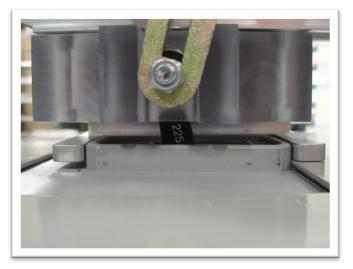
**Step 4:** If stroke adjustment is needed, loosen the 2 bolts on the front of the RSA-66A and slide outward to lengthen stroke or inward to shorten stroke. Be sure to retighten the bolts before operating the RSA-66A.
