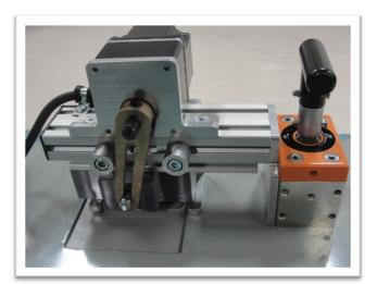
**Step 3:** Verify the switch is between the slot of the black switch adapter and the switch locator is seated flush against the base of the switch.
