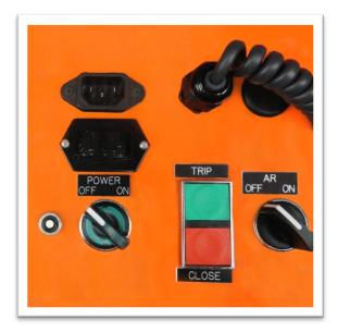
Step 6: To close, press and hold the "CLOSE" button until the breaker is closed.
