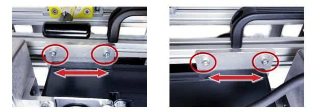
2. Slide the motor up or down to align the handle adapter with the handle on the breaker and retighten the four bolts.
