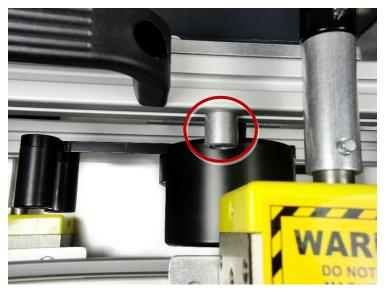
3. Move the handle and RSA operator arm fully to the end of travel in the "CLOSE" direction, then slide the travel stop until it contacts the RSA arm as shown.
