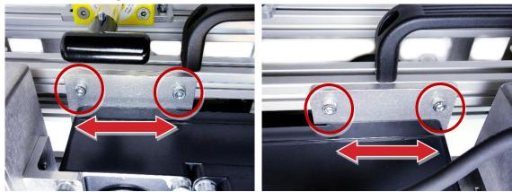
2. Slide the motor up or down to align the handle adapter with the handle on the breaker and retighten the four bolts.
