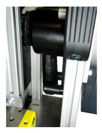
5. To attach the RSA to the breaker turn the handles of the twist-lock magnets 180° clockwise.
