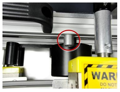
3. Move the handle and RSA operator arm fully to the end of travel in the "CLOSE" direction, then slide the travel stop until it contacts the RSA arm as shown.
