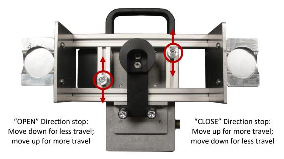
**Step 2**: Another adjustment which may need to be made is the location of the RSA-80A motor assembly. Adjusting the motor assembly may be necessary in the event that a magnet or other component on the RSA interferes with a component on the breaker or door. See the following image for directions on adjusting the motor assembly location on the RSA-80A frame.
