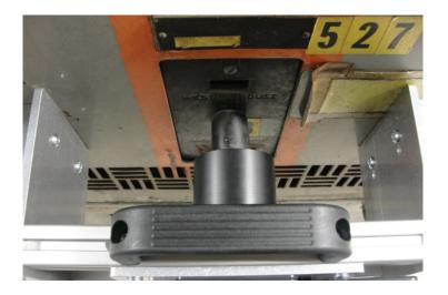
Step 4: Next, secure the RSA-80A into place by rotating the handles of each of the two twistlock magnets 180° clockwise.
