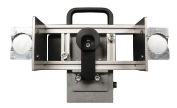
**Step 3**: Install the RSA-80A on the breaker by resting the black delrin portion of the handle adapter on the CLOSE/TRIP handle of the breaker and position the RSA so that the magnets are sitting flush against the surface of the door. See image below for details.
