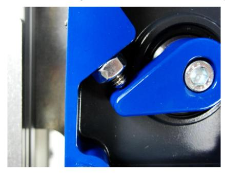
4. Move the charging handle and RSA operator arm fully to the CHARGED position, then screw in the travel stop until the stop contacts the cam as shown. Tighten the lock nut afterwards to hold it in place
