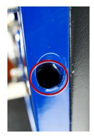
3. With the charging handle and RSA operator arm fully at rest, screw in the resting travel stop towards the stop cam until it contacts as shown. Tighten the lock nut afterwards to hold it in place.
