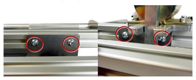
2. Slide the operator up or down as required to achieve proper alignment.
