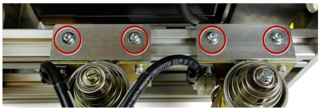
2. Slide the solenoid assembly as required to properly align the solenoids with the breaker pushbuttons, as described in the Installation section.
