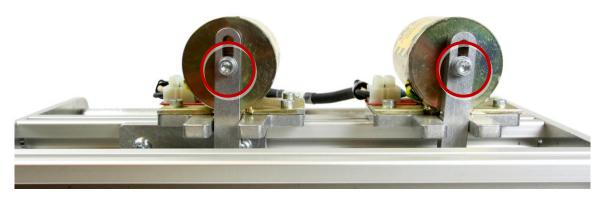
2. Slide the solenoid arms out or in as required to properly align the solenoids with the breaker pushbuttons, as described in the Installation section.
