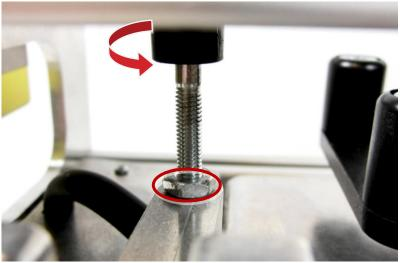
2. To decrease the solenoid plunger depth, loosen the nut on the solenoid plunger, and turn the black end clockwise. Test the depth by operating the appropriate plunger with the RSO, and re-tighten the nut.
