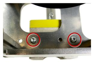
2. Move the magent to the next set of holes that will permit the RSA to be installed without interference.
