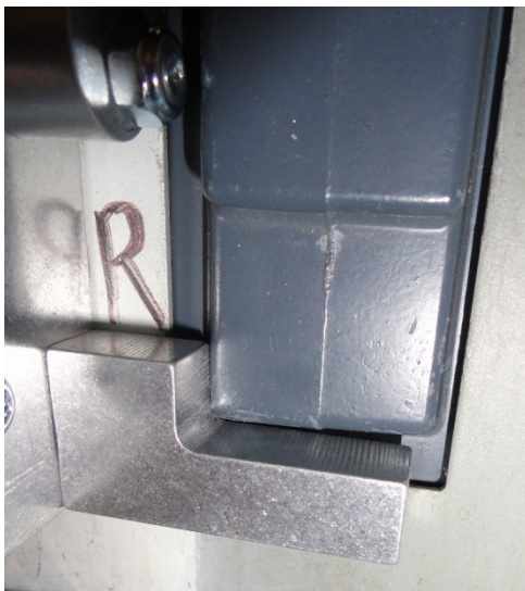
Step 5: Ensure the bottom support of the RSA-99 is positioned against the bottom of the switch.
