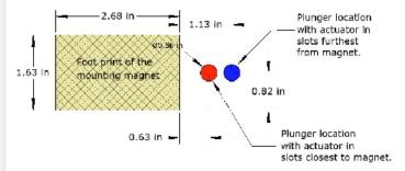
With the plunger in the retracted position, the actuator can be infinitely adjusted so that the plunger is anywhere from 0.30" to as much as 1.40" above the magnet mounting surface (which is normally the surface of your equipment). The plunger can extend up to 2". Therefore, in the lowest position (0.30"), the plunger can push into a recessed hole as far as 1.70". In the highest setting (1.40"), the plunger can push into a recessed hole as far as 0.60"
