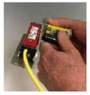
**STEP 2:** Determine which slots that the plunger should be in for your application and adjust plunger to those slots. Also, determine the starting height of the plunger and tightened the thumbscrews.
