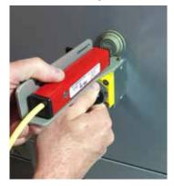
**STEP 5:** At this point the actuator should be firmly attached to the switchgear door with the plunger tip over your button.
