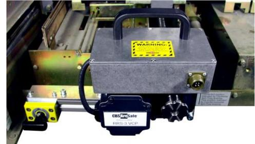
Installation and operation of the CBS ArcSafe RRS-3 VCP is quick and simple and does not require any modifications to the existing equipment. VCP-style circuit breakers typically may be found in industrial plants, utility and co-generation facilities, and commercial and residential buildings. By automating the racking procedure, the CBS ArcSafe RRS-3 VCP reduces operator fatigue and increases operator safety.
