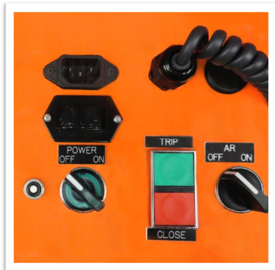
Figure 5: RSO-I control panel
