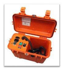
**Step 3**: Remove the cable from the cord storage area inside the RSO and connect the cable to the corresponding receptacle on the RSA-174E. Once the RSO-I AR has been connected, exit the arc flash boundary
