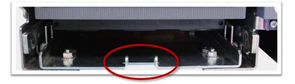
**Step 4:** The two black delrin locators should rest inside the outer steel tabs to keep the RSA-174F from moving side to side as shown in the image below.
