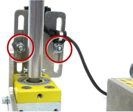
3. Slide the motor mount toward or away from the face of the Breaker Control Switch until the handle adapter is fully seated inside.
