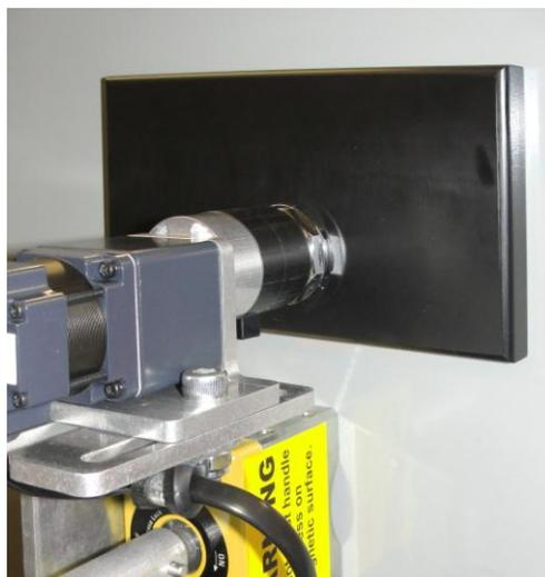
4. Turn the handles of the twist-lock magnet 180° clockwise to hold the RSA in place.
