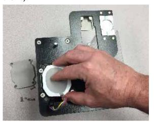
**STEP 5**: The battery connector should be in the space provided as shown below
