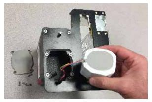
**STEP 4**: Plug new battery into the connector and slide battery into place. NOTE: The battery will only go in one way.
