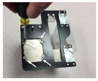
STEP 2: Remove battery cover plate and slide battery out.
