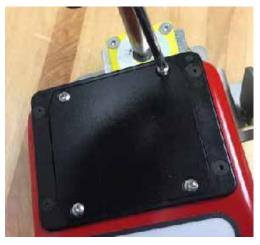
**STEP 2**: Remove battery cover plate and slide battery out.
