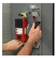
**STEP 2**: While firmly holding the actuator in your right hand, disengage the magnets by using your left hand to turn the magnet lever counter-clockwise. Lower the actuator off the operating handle.
