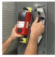
**STEP 3**: Disconnect cable (for cabled versions only) and return components to carrying case or store on the side of the MCC. (See Section 5.0 for details)
