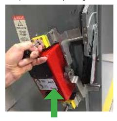
Use a similar (reverse) action when the disconnect handle is in the UP position. Start at the top, slipping the actuator arm behind the disconnect handle. Rotate the RSK-ABL3 downward.
