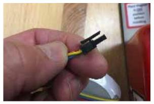
**STEP 4**: Plug new battery into the connector and slide battery into place. NOTE: The battery will only go in one way. The end where the battery leads exit the battery must go in first.
