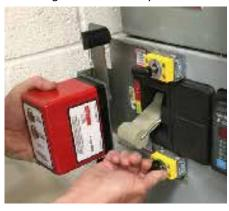
**STEP 5:** Turn the RSK-CHL1 ON by pressing the WAKE button. The light on the button should illuminate and stay lit. If light flashes and turns off, it is an indication that the batteries need to be replaced. You will need to replace the batteries in the hand-held controller and then repeat this step.
